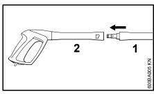
Press the spray lance (1) into the mount on the spray gun (2), turn it by 90° so that it engages
