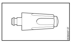
Nozzle with rotating jet. To remove stubborn dirt on hard-wearing surfaces. Maximum effect at a distance of 10 cm.
