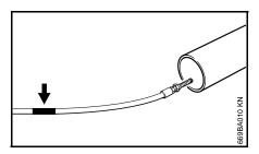
There is a mark on the cleaning hose underneath the nozzle (see arrow).
