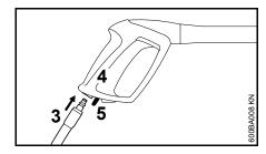
Push the connector (3) of the highpressure hose into the mount on the spray gun (4) until it engages
