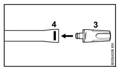
Insert nozzle (3) in spray lance until the safety latch (4) engages – at which point the safety latch button will spring out again – the adjustable high-pressure nozzle has an antitwist device; orient this according to the groove on the spray lance
