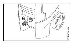
Attach the connector (6) to the water inlet by hand and tighten it
