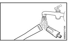
Rinse the connection latches of the spray lance and nozzle with water so that no deposits form
