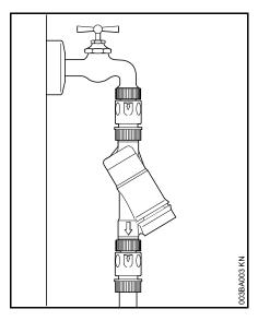
When hooking up to the drinking water main, a backflow preventer must be installed between the water tap and the hose. The design of the backflow preventer must comply with the applicable country-specific regulations.
