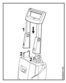
Press the handle frame (1) onto the holders (2) from above – handle frame must snap into position
