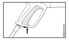
Press the safety latch – the lever is locked to prevent inadvertent operation
